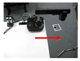
2) To remedy this situation, rotate the camera head by swinging it down and around (clockwise).
