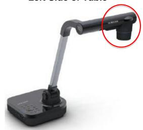
• If you have placed the doc cam in the left hand corner of the table, the doc cam lens will be turned so that the camera lens itself is to the right of the base. See the picture here. This allows the camera head to be positioned on the presentation station table and provides room to place documents and object underneath.
